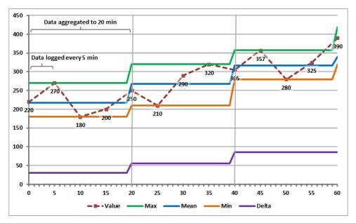
Figure 24: Aggregation of plant data
